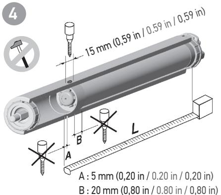
**3****FR Installer le tube sur ses supports****EN Install the tube on the brackets****IT Montare il tubo sui propri supporti**
