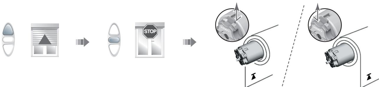
**5****FR** Paramétrage du fin de course bas**EN** Down limit adjustment**IT** Configurazione del finecorsa inferiore
