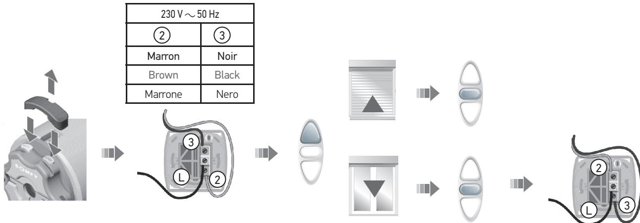
**FR** Paramétrage du fin de course haut**EN** Up limit adjustment**IT** Configurazione del finecorsa superiore
